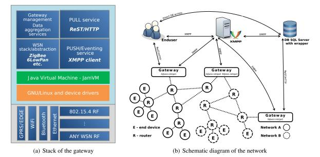
Figure 2: Software building blocks and schematic diagram of the network
